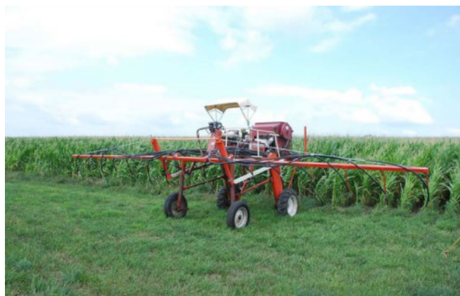
Figure 7. A high-clearance sprayer modified to seed cover crops into standing corn. Image courtesy of Sarah Carlson.
